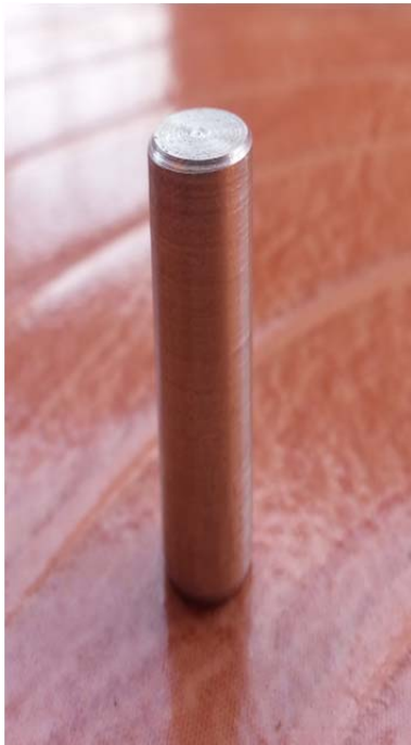
Fig. 1. a) wear test specimen (b) Pin on Disc wear setup
